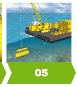
Tunnelling machine is prepared for release from pipestring; bulkhead is closed
